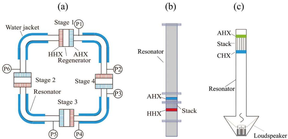
Fig. 1. Some examples of thermoacoustic systems. (a) A dry travelling-wave engine (adapted from Jin et al. [17].) (b) A wet standing-wave engine (adapted from Brustin et al. [18].) (c) A wet standing-wave refrigerator (adapted from Yang et al. [10]). AHX-ambient heat exchanger, HHX-hot heat exchanger, CHX-cold heat exchanger.
