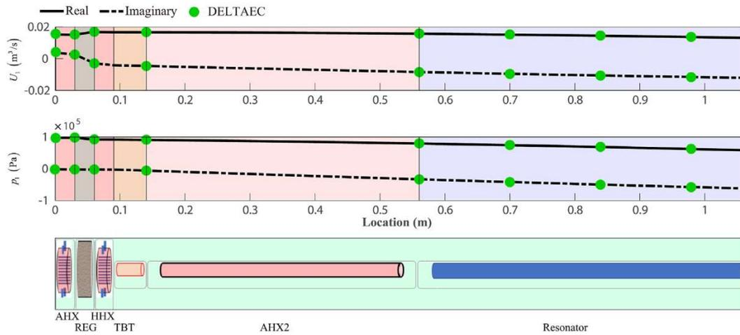
**Fig. 3.** Distributions of the volumetric velocity amplitude (top) and the pressure amplitude (middle) in the travelling-Wave engine designed by Jin et al. [17]. Schematic of the engine generated by PC-TAS is displayed at the bottom. Note that the resonator is only partly shown, because it is too long.
