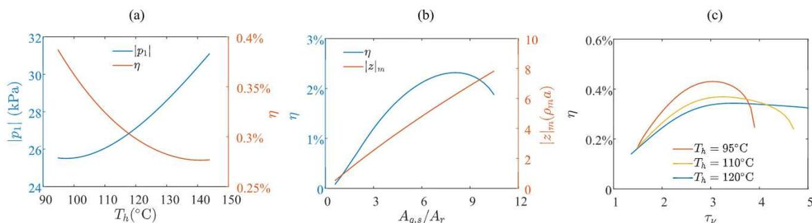
**Fig. 5.** Calculated results: (a) The pressure amplitude  $|p_1|$  and the efficiency  $\eta$  vs. the hot temperature  $T_h$ . (b) The influence of the area ratio  $A_{g,s}/A_r$  on the efficiency  $\eta$  and the mean acoustic impedance  $|z|_m$ . (c) The influence of the Womersley number  $\tau_v$  on the efficiency  $\eta$ . The working mixture is nitrogen and ethanol, the mean pressure is 10 bar  $\Delta T = 56$  °C.
