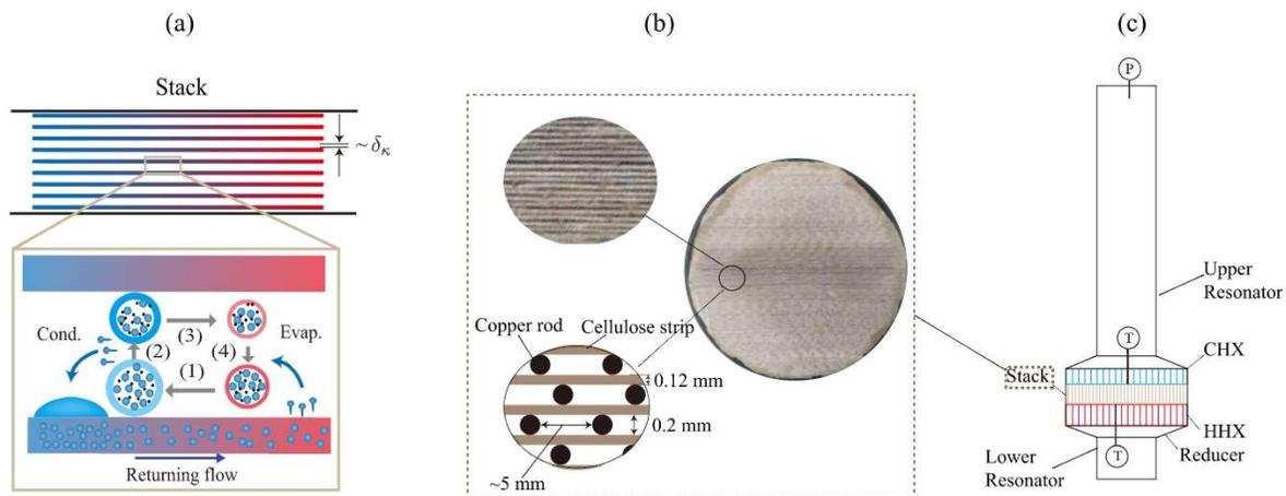
**Fig. 1.** (a) The thermodynamic cycle of the phase-change standing-wave thermoacoustic conversion: (1) adiabatic expansion, (2) isobaric heat rejection with mass loss, (3) adiabatic compression and (4) isobaric heat absorption with mass gain. (b) Structure of the stack. (c) Schematic of the phase-change standing-wave thermoacoustic engine. HHX-hot heat exchanger, CHX-cold heat exchanger. P-pressure sensor. T-thermocouple.
